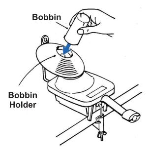
b) Move the bobbin in counter clockwise direction to fit into the bobbin holder
